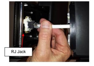
This cable connects the load cells to the display head and must be entirely plugged in for the scale to function properly.
