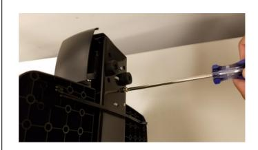
6. Locate the 2 M6 x 16mm screws included in the clear plastic bag. Align the 2 holes in the tray with the mounting holes on the scale platform. Insert the screws and tighten to attach the tray to the scale platform.
