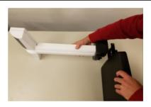
4. Locate the load cell connector cable inside the column and pull gently until the plug reaches the bottom of the column. Carefully pull the cable connector from the bottom of the column and plug into the RJ jack on the scale platform. Caution: Once connected, keep a firm grip on the columns to ensure the load cell connector cable is not pulled out from the RJ jack.
