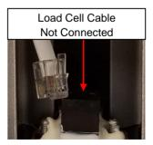
2. Inspect the load cell connector cable to ensure it is completely plugged into the RJ jack. If cable was plugged in, unplug and plug in again until it clicks into place. After checking connection, replace door at the back of the platform base.
