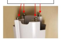
Remove the black adapter bracket from scale platform. Place the bracket on the bottom of the column with the adapter jack arrow sticker pointing towards the front of the column.
