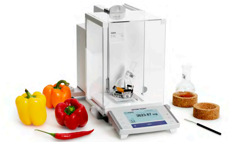
Figure 7: ErgoClip holders stabilize the tare container in the XPE and XS analytical balance to enable one-step direct dosing and therefore eliminate sample-transfer errors and scattering
