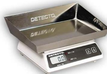
Useful for weighing very small animals, the PS5-2KD features a roomy, stainless steel tray which is removable and easy to clean. Lightweight at just five pounds, the durable PS5-2KD is powered by either four AA batteries (not included) or an optional AC adapter. An easy-to-read 1/2" (13mm) high LCD, and capacity and increments of 70 oz x .1 oz / 1,998 g x 2 g make it ideal for weighing kittens, hamsters, rabbits, lizards, and other small animals.
