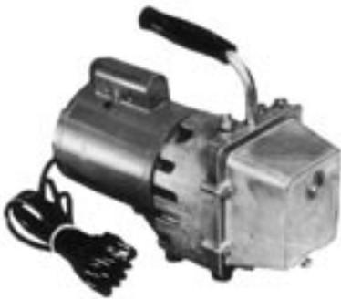
The **G8274** two stage Vacuum pump produces 1-micron of ultimate pressure while the rotary sliding vane provides 85 liter per minute (3 cfm) capacity and operates quietly. It also features a direct drive which reduces operating space needed. The gas ballast helps purge moisture from the vacuum system while the trap reduces the risk of traveling back into the system. The pump operates at 1725 RPM with a 1/2 HP 110, 60 HZ motor. Furnished complete with initial supply of High Vacuum Pump Oil.
