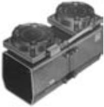
The **G8270** pump is an oilless two stage diaphragm vacuum pump that can be used with the Hogentogler vacuum pycnometers and for other applications that require a vacuum source. This pump has a rugged construction that requires very little maintenance. The pump produces a maximum vacuum of 29" of mercury and has a free air displacement of 1.15 CFM. The pump is available in both 110V/60Hz and 220V/50Hz models (please specify type needed).
